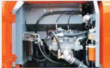
Grouped remote filters and inspection points
