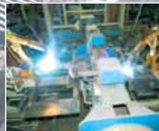
Main frame welding line
