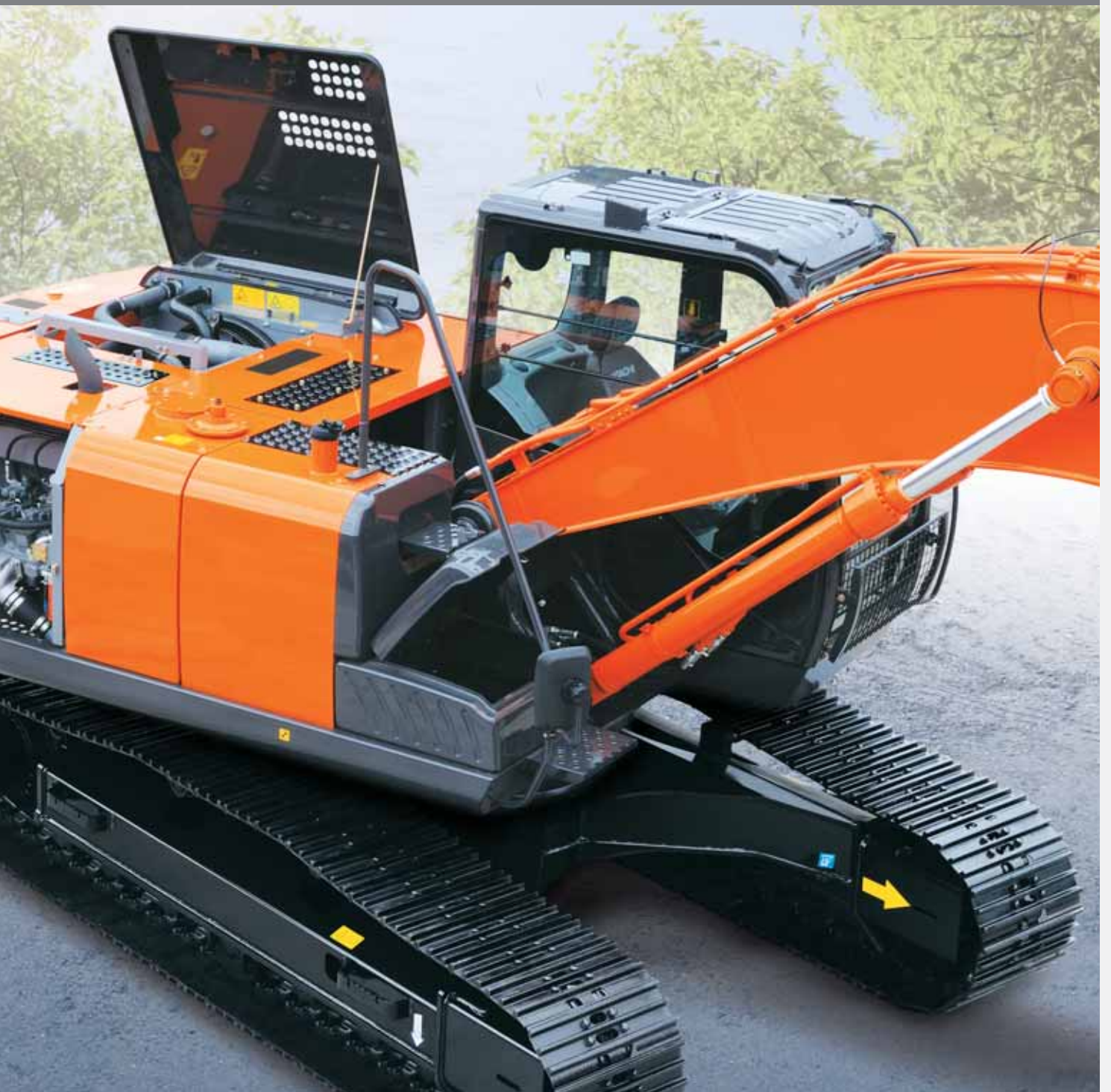
The photo shows an excavator with an optional front glass lower guard.
