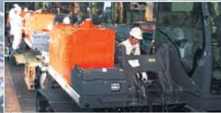
Mid-sized excavator assembly line
