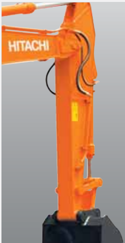
Attachment basic piping
